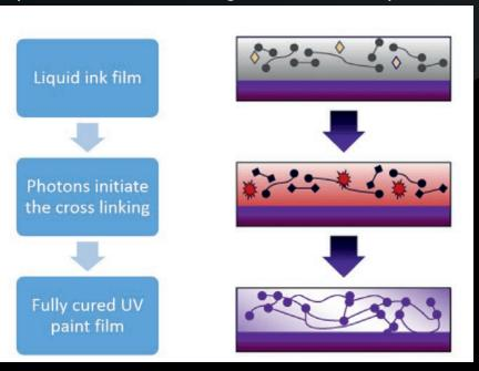
Another benefit of this application process is that when using the solid UV ink 100% of the ink remains on the substrate. With solvent-based inks, the ink deposit will shrink during the drying process until only the pigments and resins remain, leading to a less durable and less precise finish.
